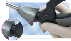
Rotate safety ring so that the opening is pointing to the lever.
