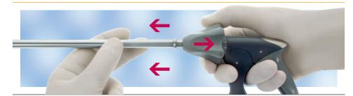
Hold instrument shaft. Pull back star wheel to disengage the safety ring and to release instrument shaft. Remove safety ring from handle.
