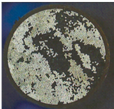
Fig. 2 Damaged light guide fibers
