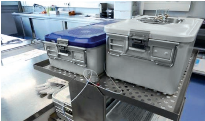
Positioning of thermal elements to evaluate the sterilization performance of PRIMELine® PRO and Basic container systems.
