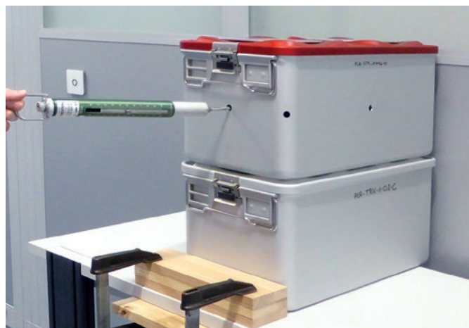
Performing a stacking tensile test with PRIMELine® PRO.
