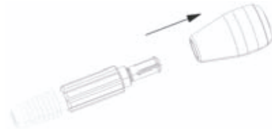
Fig. 8 Disassembling of twist drill handle
