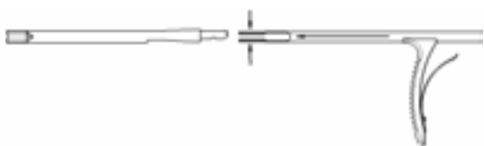
Fig. 13 Assembling of rod persuader
