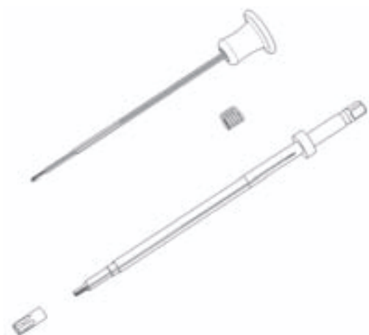
Fig. 10 Exploded view of S 4 Cervical self holding polyaxial screwdriver
