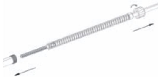
Fig. 9 Disassembling of taps
