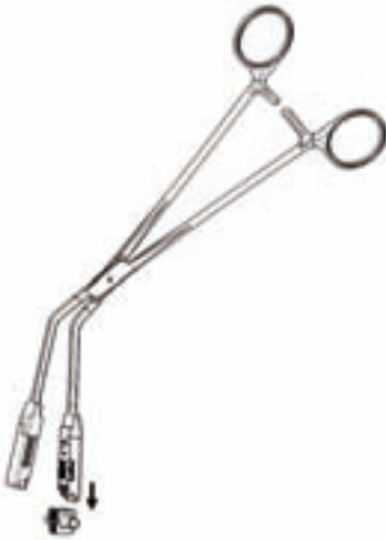
Fig. 1 Inserting the spring element in the insertion pliers
