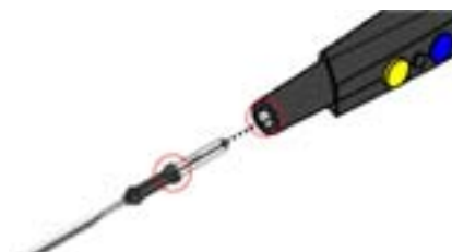
Fig. 5 Inserting the working electrode in the handle
