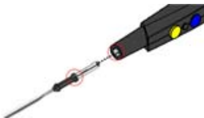
Fig. 5 Inserting the working electrode in the handle
