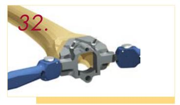
The drilling guide for the  $\emptyset$  14 mm drill is applied so that its peg fits into the lower central hole of the PS preparation guide.
