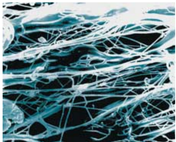
Lyophilized Lyoplast ® (Magnification 4000 x). Loosely connected skeins of collagen fibres, which are surrounded by a network of fine fibres.
