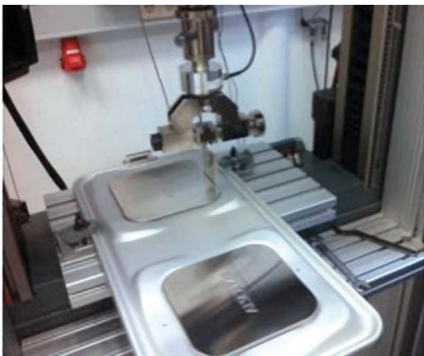
Extractor Testing of the exterior stainless steel cover.
