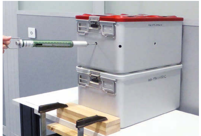
Performing a stacking tensile test with PRIMELine® PRO.
