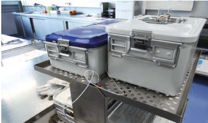
Positioning of thermal elements to evaluate the sterilization performance of PRIMELine® PRO and Basic container systems.
