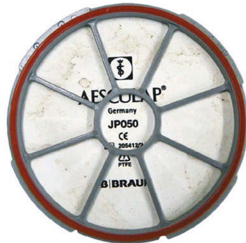
Discolored filter disc due to the impact of repeated reprocessing.
