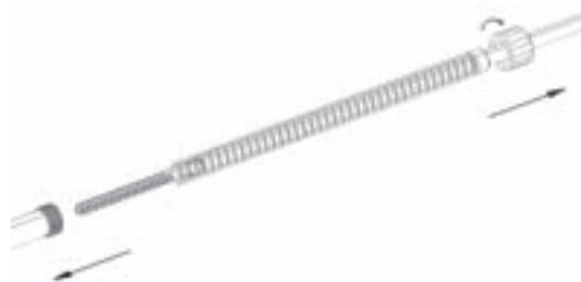
Fig. 9 Disassembling of taps
