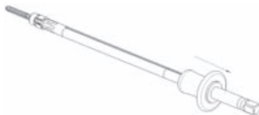
Fig. 6 Picking up the S 4 Cervical screw
