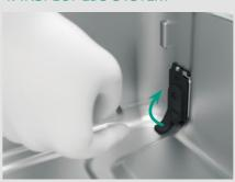
I Remove condensate outlet for inspection.
