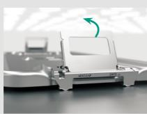
Locking mechanism fully functional. Check for dents and deformations.
