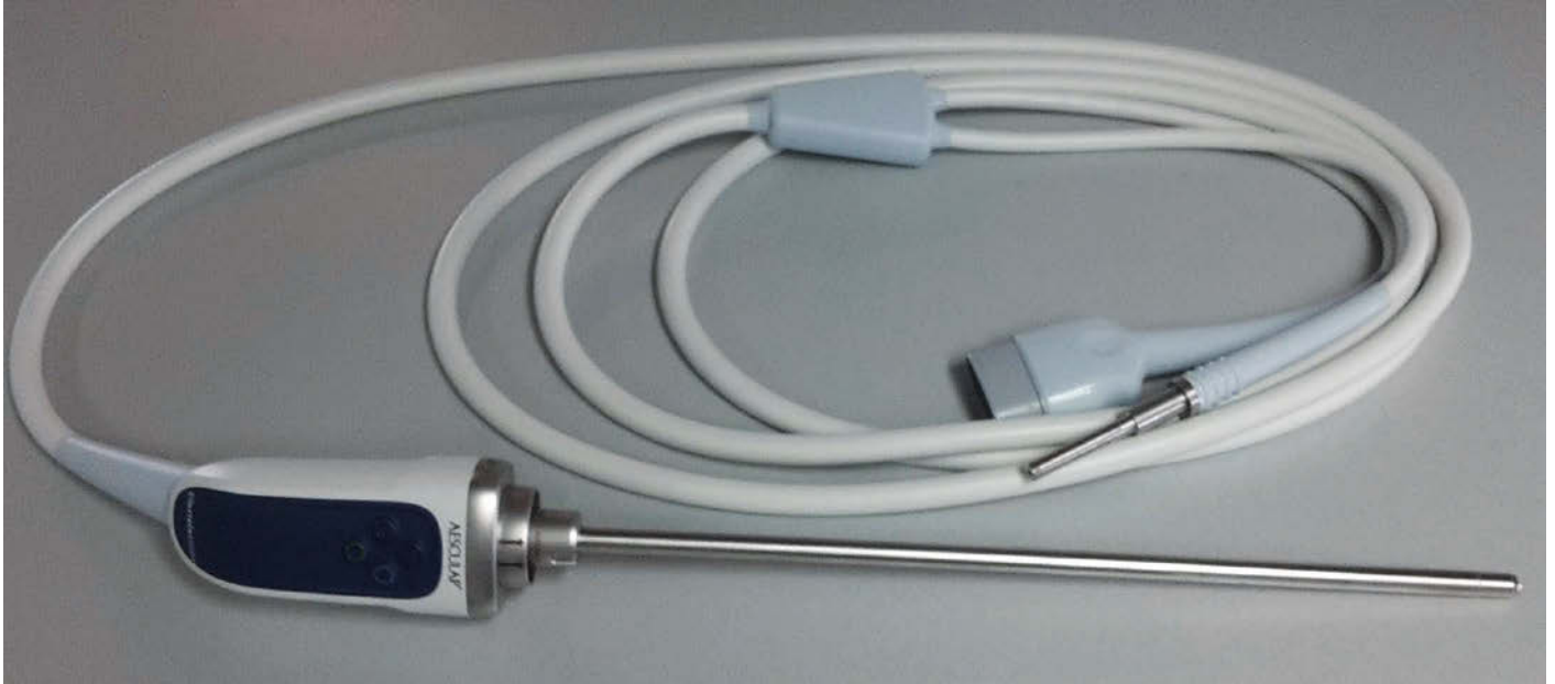
Fig. 7: Camera head with cable and plug (Item 160)
