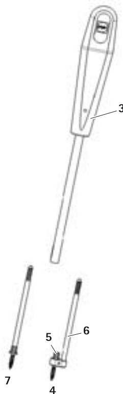
Fig. 1 Distraction screwdriver with distraction screw and offset distraction screw
