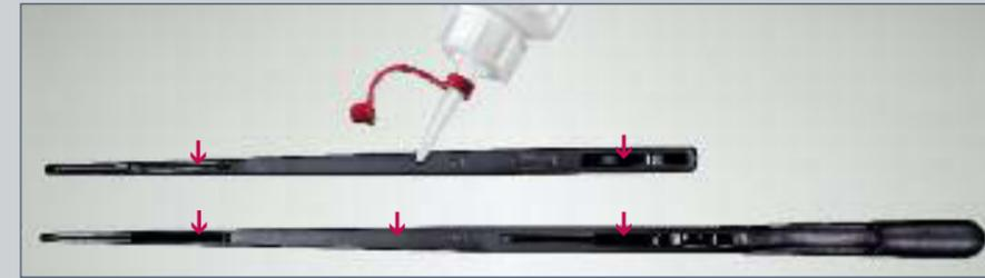
Lubricate the defined places on the instruments with Aesculap® STERILIT® Oil e. g. JG598 after each cleaning cycle.
