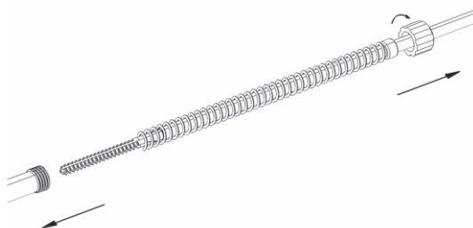
Fig. 9 Disassembling of taps
