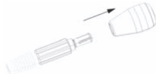
Fig. 8 Disassembling of twist drill handle
