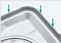
No dents in rim of the container lid Aluminium lid not warped
