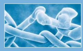
The use of thin monofilaments and a hightechnology knitting process makes it possible to produce a thin mesh which greatly improves the trimming and handling during implantation. The thin mesh is characterized by its high elasticity and its fine polypropylene monofilaments.
