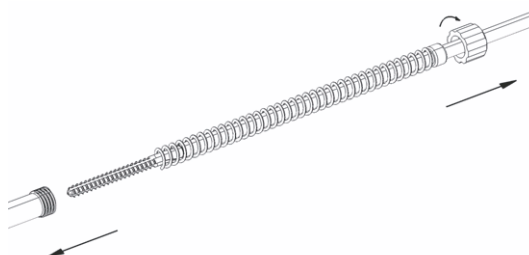
Fig. 9 Disassembling of taps
