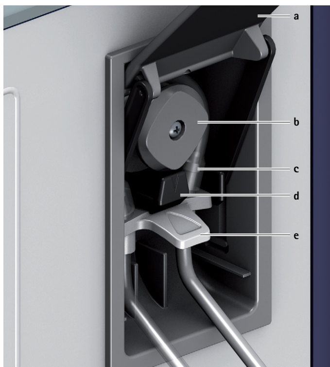
Fig. 4 Connecting the single-use tube set
